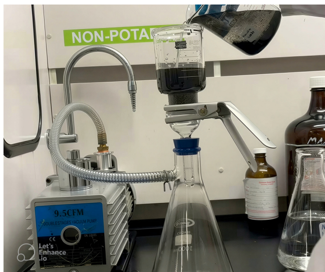
Fig. 1 — Vacuum-assisted Buchner filtration setup: 9.5 CFM double-stage vacuum pump (left), filtration funnel with graphene suspension being poured in, and 1000 mL Erlenmeyer flask collecting the filtrate. This setup was used across multiple purification cycles to isolate the graphene-rich fraction from electrolyte residuals.
