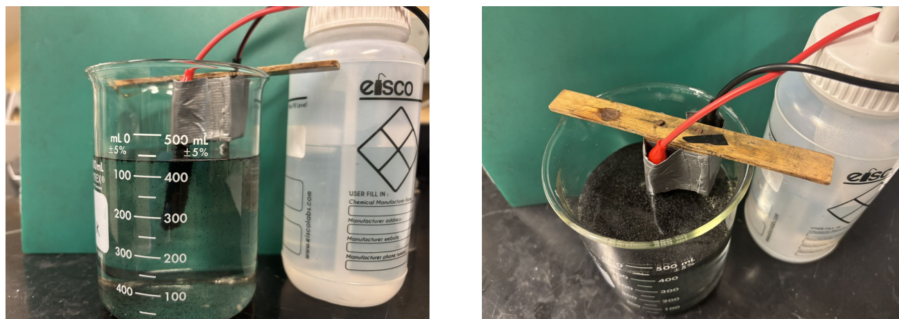
Fig. 2 — Left: graphite anode and cathode submerged in ammonium sulfate electrolyte during an early-stage exfoliation run, electrolyte still relatively clear. Right: dense graphene nanoflake suspension visible after extended exfoliation, solution turned deep black as material separated from the graphite anode.
