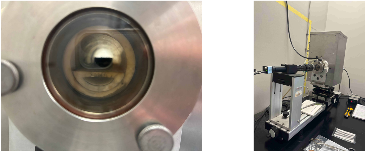
Fig. 2 — Left: interior view of the tensiometer furnace chamber showing the molten electrolyte droplet sitting on the carbon substrate plate at high temperature. Right: the full high-temperature tensiometer/furnace system (IDS camera + HTFC 1700 controller) used for all wettability trials.
