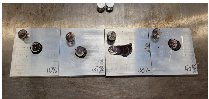
Fig. 2 — Left: adhesion strength (psi) for Bio-oils 1–4 at room temperature (Week 5, blue) vs. thermally cured at 170°C (red). Thermal curing produced roughly 10–30x strength gain across all candidates. Right: post-pull dolly plates from FeO hybrid tests at 10, 20, 30, and 40% FeO
