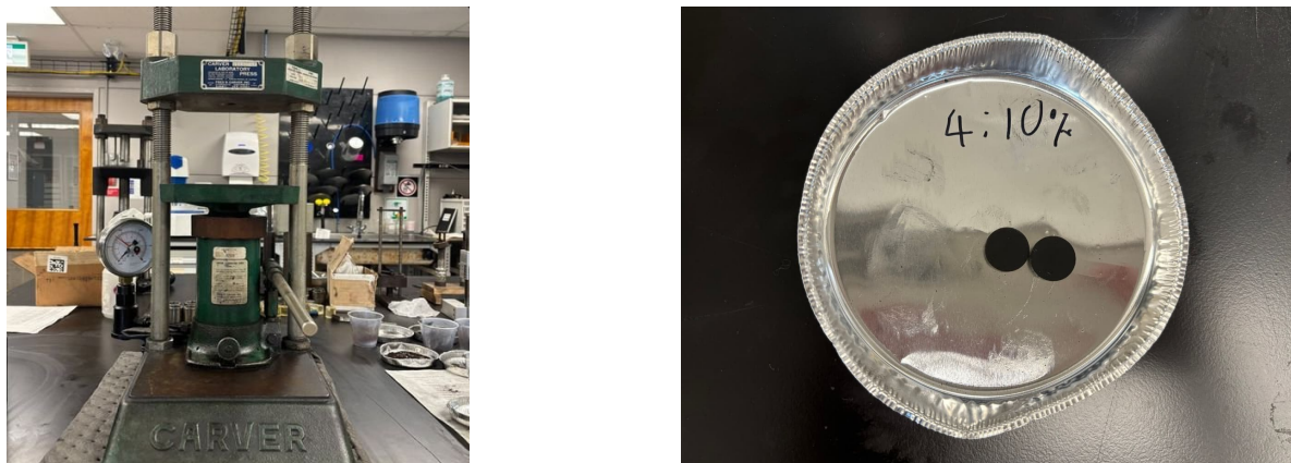
Fig. 5 — Left: Carver laboratory hydraulic press used for pellet fabrication at controlled pressure. Right: two pressed biocarbon pellets (Bio4, 10% FeO loading) after thermal curing at 140°C — maintaining visual integrity and uniform geometry post-cure.
