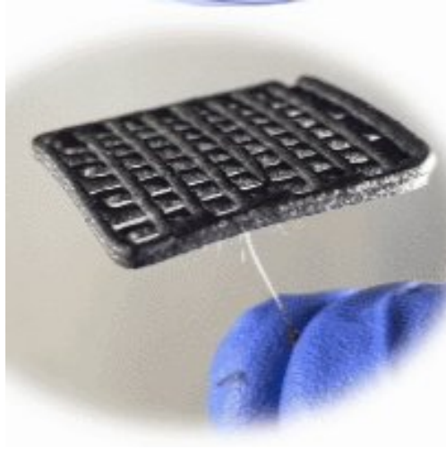
Fig. 1 — Finished cellulose aerogel scaffold held for scale, showing the open-cell grid geometry and ultralow density of the freeze-dried structure. The mechanical integrity after lyophilization confirmed successful pore preservation through the flash-freeze and sublimation process.
